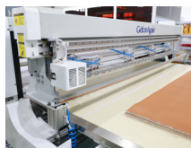
切刀自动提升装置 Automatic Cutter Lifting Device
